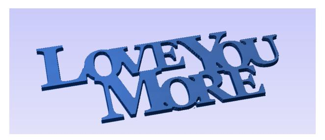
The last step in this program is to save the toolpath for the STEPCRAFT. To do this, select the toolpath you just created and click Save Toolpath(s) to File. Select the "Mach2/3 Arcs (mm) (\*.txt)" post processor from the drop-down list and save the file.
